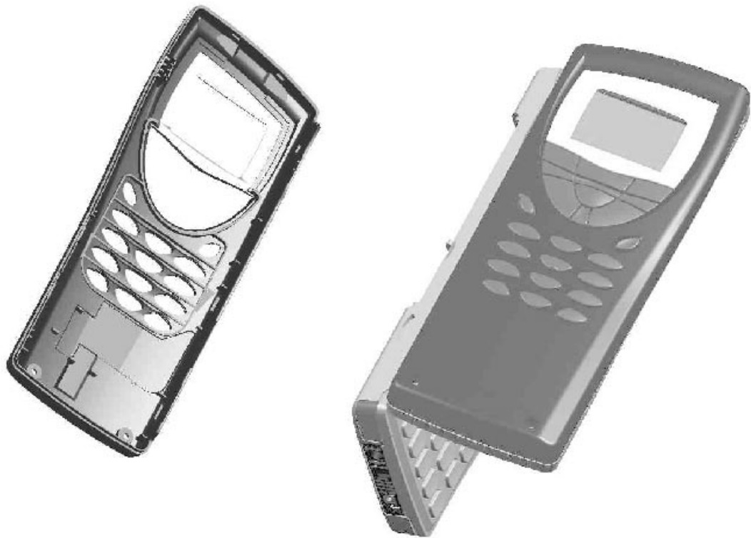
Figure 3. Remove the front cover assembly from the Screen frame.
