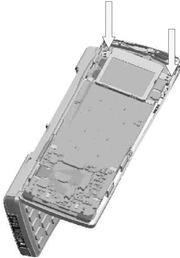
Figure 5. Remove the 2 screws from the Screen Frame.
