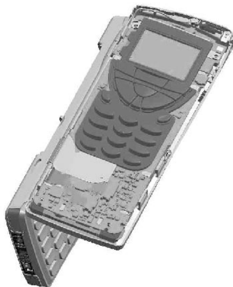
Figure 4. Remove the CMT keymat from the UI module.
