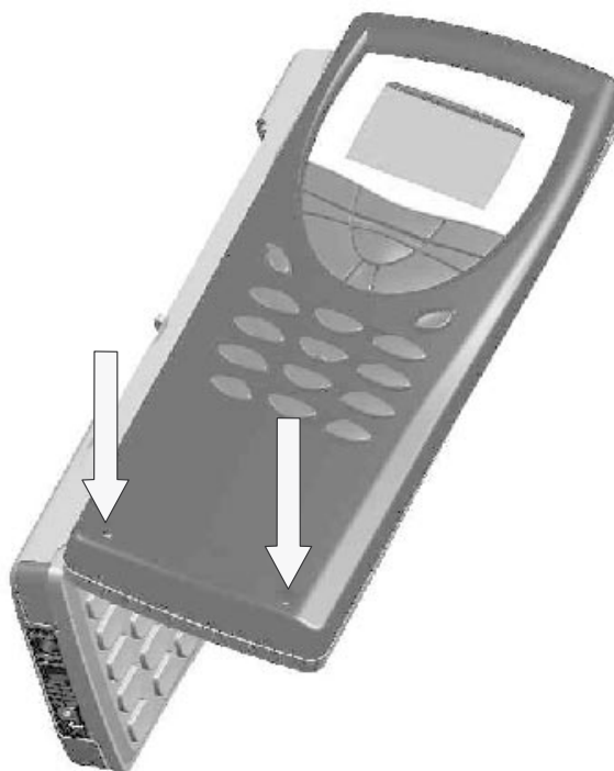
Figure 2. Remove the 2 pcs screws from the front cover assembly
