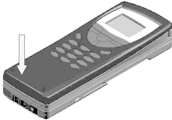
Figure 1. Remove the cover label from the front cover assembly
